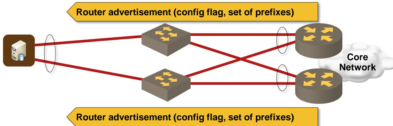
RA timers can be adjusted on most routers and L3 switches
