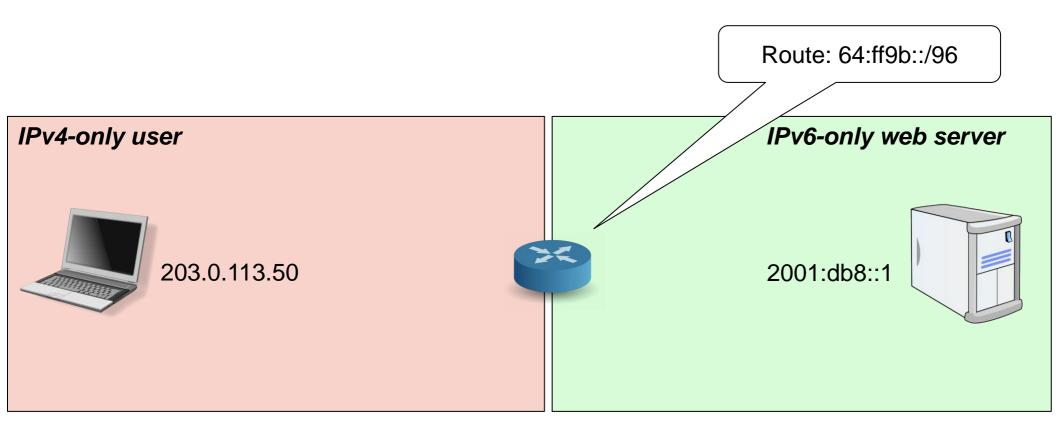
An IPv6 /96 prefix is assigned as the translation prefix representing the IPv4 internet and routed to the SIIT gateway
