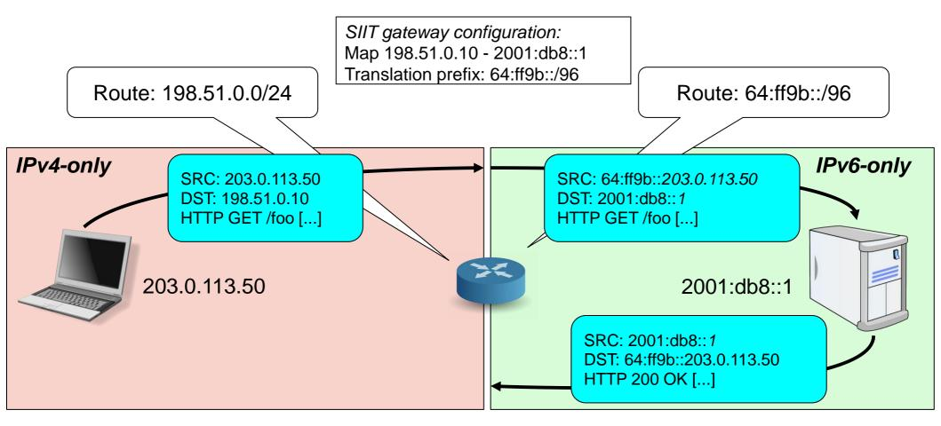
The server responds to the packet just as it would with any other IPv6 packet
