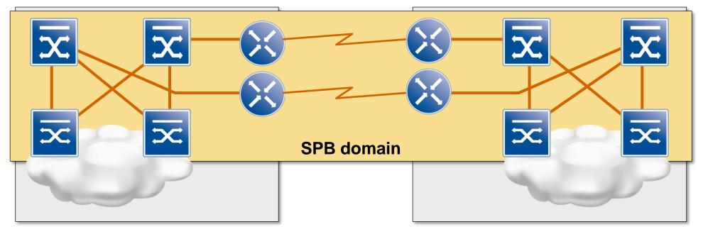
Spanning tree and MLAG/LACP replaced with SPB(V)
