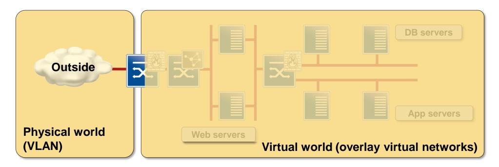
Overlay networks simplify physical network design, deployment and operations (and increase the complexity of the hypervisor software)
