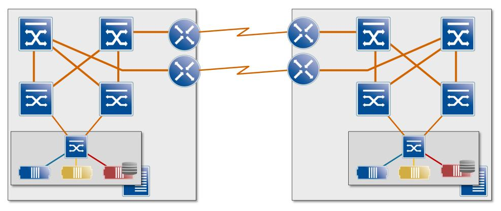
L3 interconnect: pure IP routing L2 interconnect: VLANs stretched between locations
